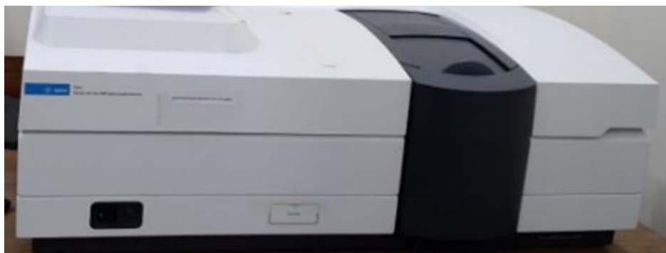
Figure 2.3.9: Schematic diagram of a UV-Vis spectrometer to check the transparency of the hydrogel
