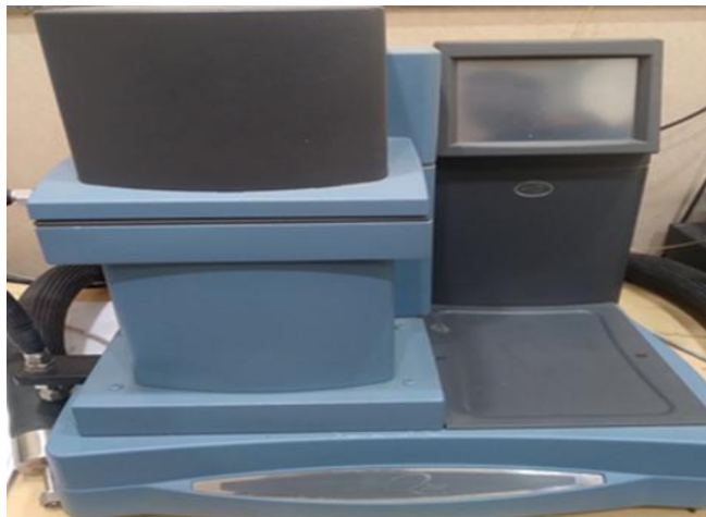
Figure 2.2.2: Schematic diagram of the Dynamic Mechanical Analyser for testing the strength of the hydrogel
