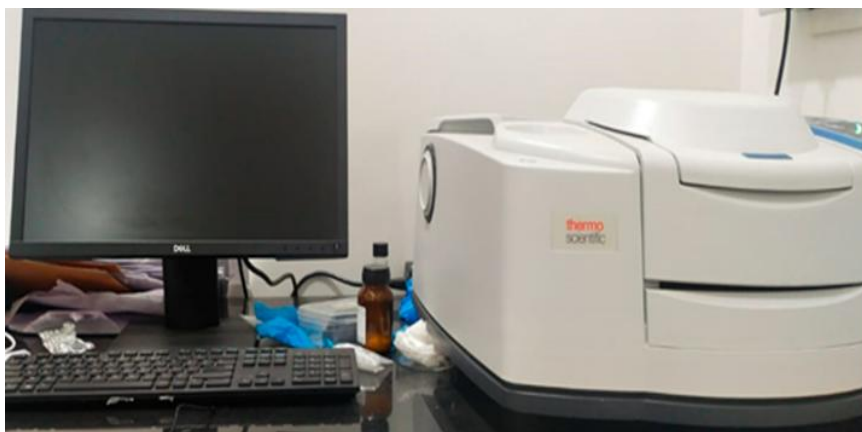
Figure 2.3.6: Schematic diagram of a Fourier Transform Infra-red spectrometer for functional group analysis
