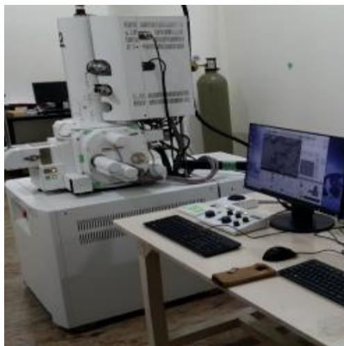
Figure 2.3.4: Schematic diagram of FE-SEM instrument for morphological study of hydrogel surface
