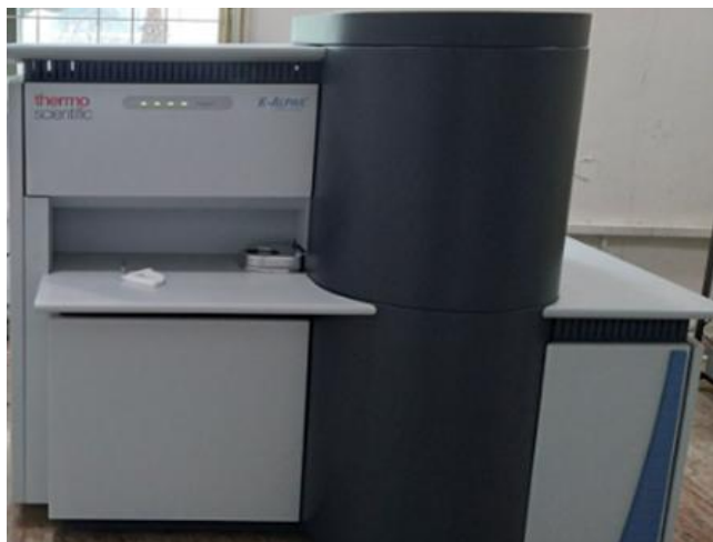
Figure 2.3.3: Schematic diagram of X-ray Photoelectron Spectrometer for elemental analysis of hydrogel
