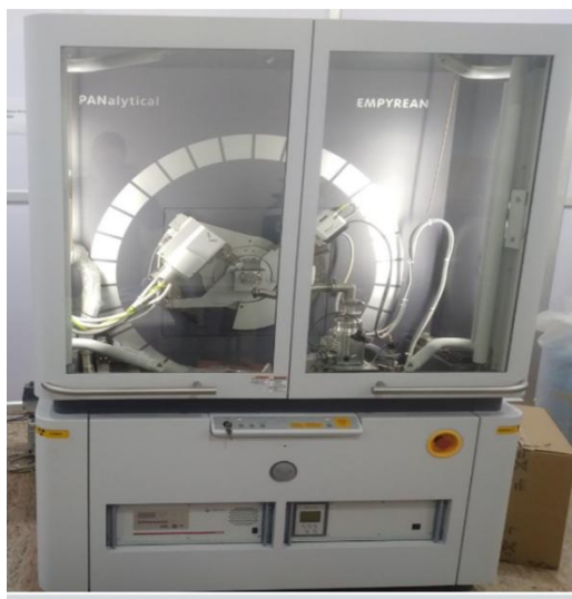
Figure 2.3.1: Schematic diagram of X-ray Powder Diffraction instrument to check crystallinity of hydrogel.
