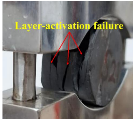
Figure 6.10. Characteristic layer-activation failure of the Krol Shale under BTS test.
