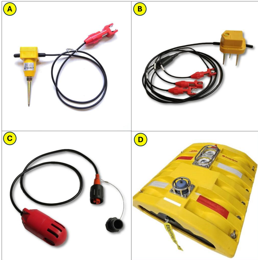
Figure 4.10: Land and Marine seismic energy receivers: (A) Geophone (B) 3C Geophone (C) Hydrophone (D) Multicomponent Geophone or ocean-bottom nodes (OBNs) (Bjorlykke, 2010).
