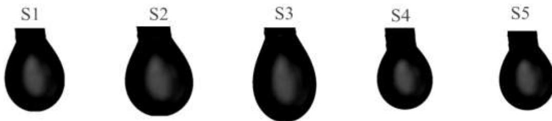
**Figure 7.8:** Actual images of the nanofluid droplets in CO<sub>2</sub> environment obtained using Phantom VCC camera and adjustable height arrangement.
