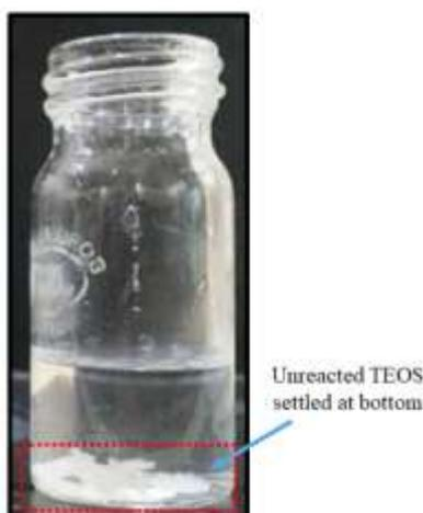
**Figure 2.4:** Effect of high PAM concentration (2000 ppm) on synthesis of silica NPs. With 2000 ppm PAM, interaction between TEOS and  $\text{NH}_3$  led to white globules (instead milky appearance) those eventually settled at the bottom.
