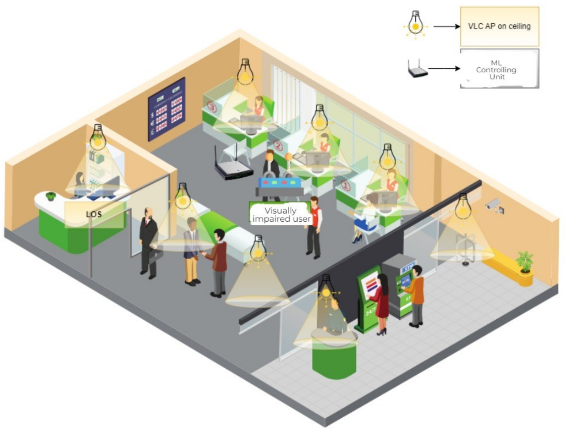
Figure: A schematic diagram illustrating a typical scenario under consideration with a visually impaired person in a public place with light sources.
